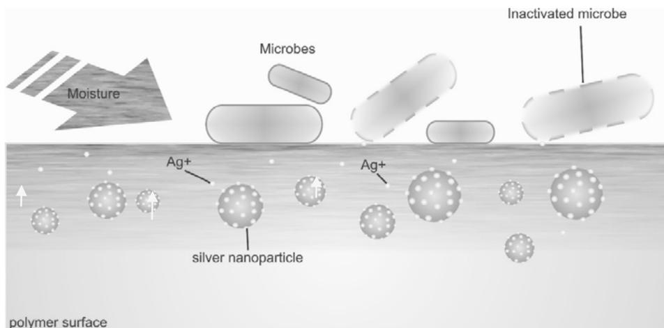
Figure 1: Schematic overview of the nanosilver effect on surfaces (© RAS AG)
