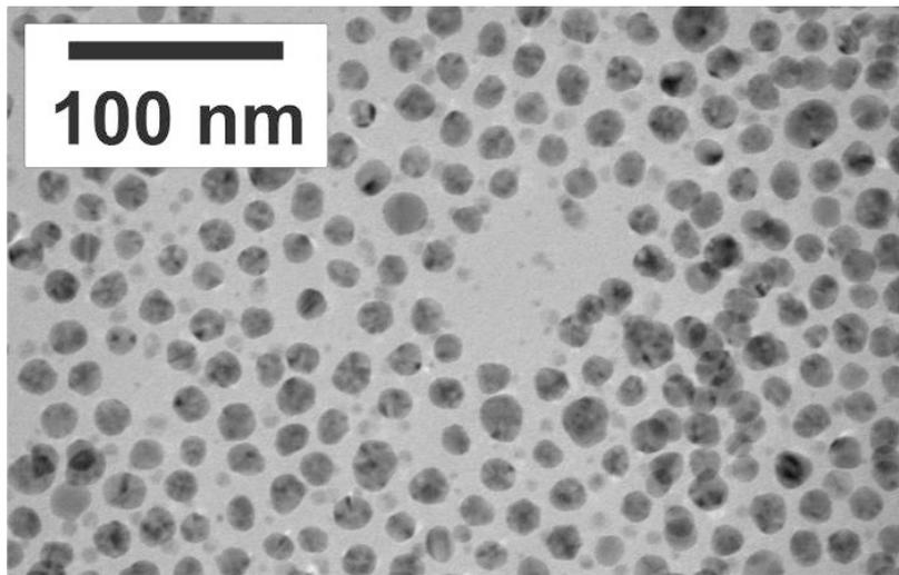
Figure 3: TEM-image of NM 300K (= agpure W10, a product of RAS AG) nanosilver particles. (Klein et al. 2011 [17]).
